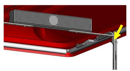
DRILL 5/16" DIAMETER HOLES THROUGH TOP SUPPORTS OR TOP RAILS AND MOUNT WITH HARDWARE SUPPLIED.
