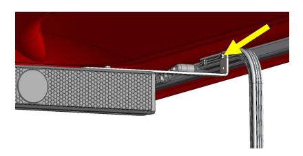
MOUNT ASSEMBLY TO AN EXISTING HOLE LOCATION UNDER THE CANOPY.
